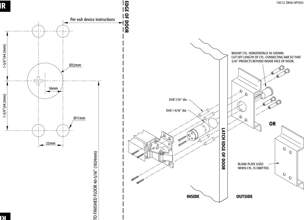
EDGE OF DOOR Per exit device instructions 1-3/4"(44.5mm) Ø32mm 2-5/32x5/8" \[\] 16mm OR 1-3/4"(44.5mm) Ø11mm 0 OR LATCH EDGE OF DOOR  $\mathcal{O}$ 22mm BLANK PLATE USED WHEN CYL. IS OMITTED. TO FINISHED FLOOR 40-5/16" (1024mm) **OUTSIDE INSIDE**
