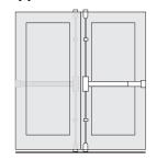
**2 Vertical Rod type.** Double egress surface applied. 2 point locking both doors opposite directions.
